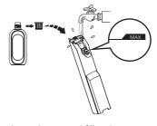
Open the tank cap, and fill with tap water to the Max line. When deep cleaning is necessary, add one bottle cap of solution to the CWT and tightly close the cap.
